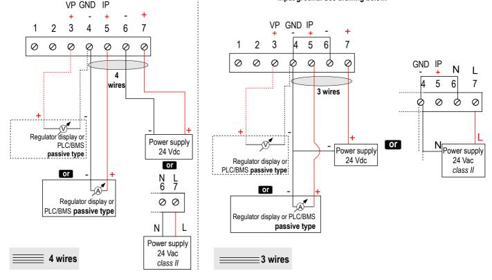
For CP112/113 - PO models and CP112/113 - PN models with 4-20 mA output - passive :
